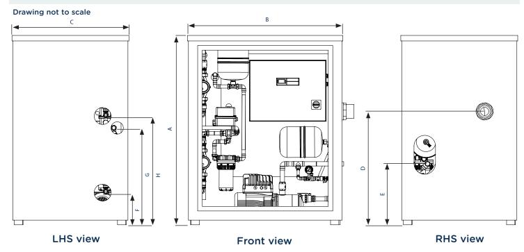
Unit must be installed at least 100mm away from a solid surface to enable the type 'AB' airbreak to function correctly at the back of the unit.
